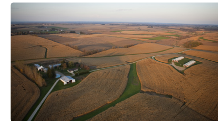
Grassed waterways in the Root River watershed in southeastern Minnesota prevent soil erosion while draining runoff water from adjacent cropland.
